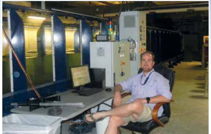
Dr. Bret Webb, Associate Professor of Civil Engineering, shows off the wave flume, which is much longer than it is wide, with a mechanical wavemaker on one end, and the construction being tested on the other end. The side walls have glass to allow for observation of the experiments.
