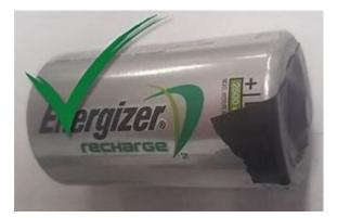
Pictures showing how battery terminal are to be taped for safety.
